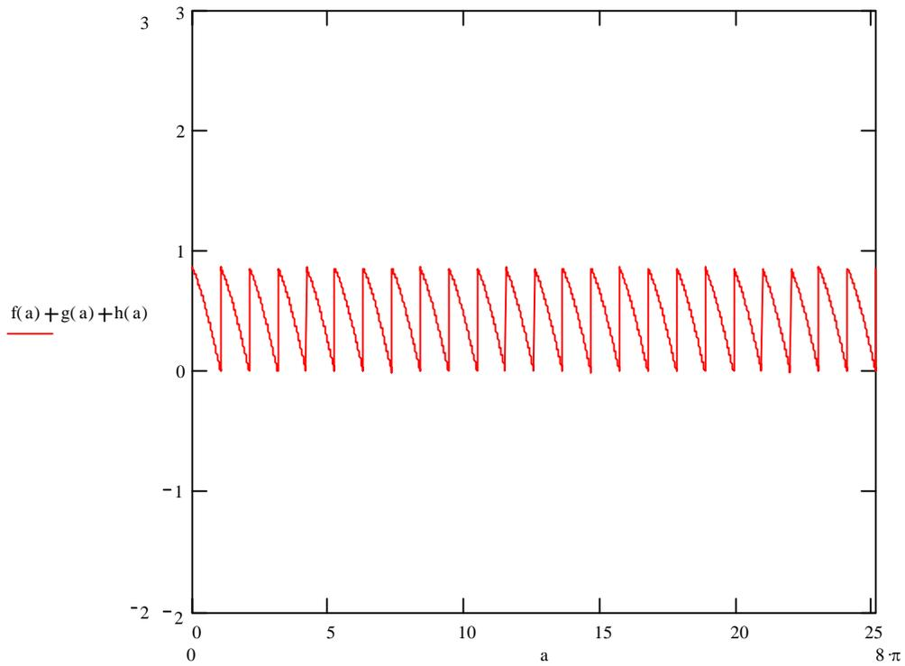
Notice that at 120 degrees, the base of the waveform (the sum of the three rectified phases) is at zero.
