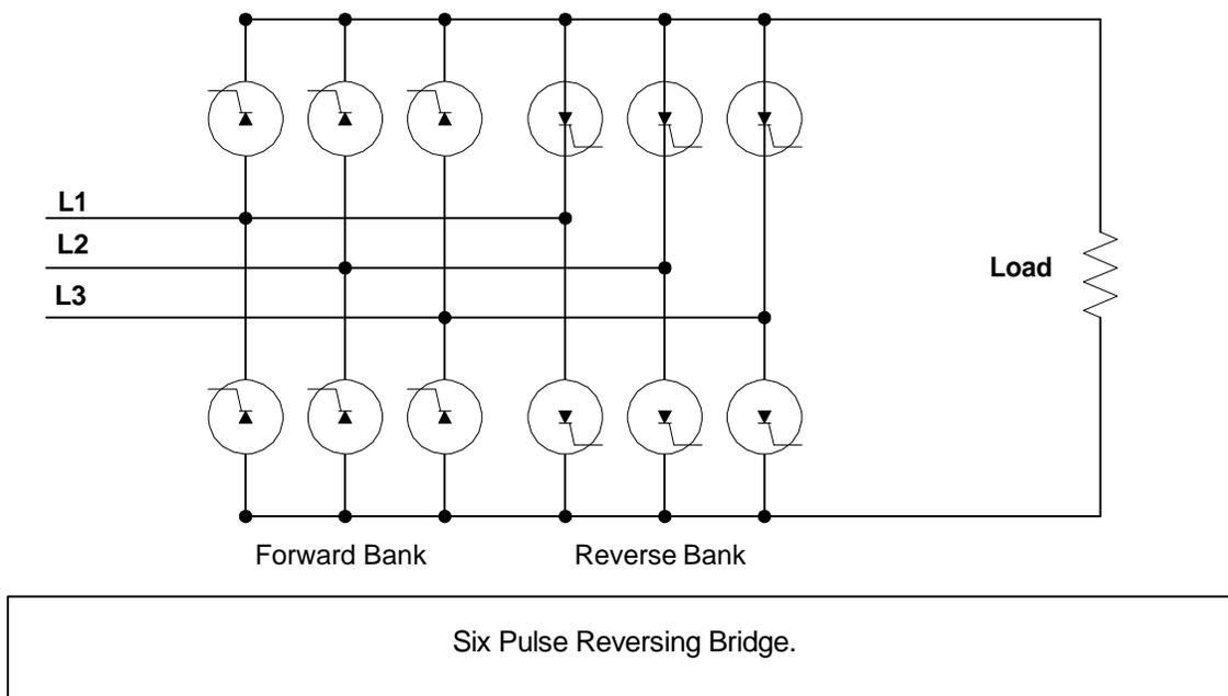
The figure above illustrates a six pulse reversing SCR phase angle controller. When the gates on the forward bank are activated, the current flow through the load is clockwise. When the gates on the reverse bank are activated, the current flow through the load is counter-clockwise. The firing angle controls the effective voltage thus the current through the load.
